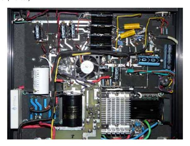
The anode voltage was chosen to be 360V (factory setting is 460V with an input network of 230V). With this choice of anode voltage, I tried find a reasonable compromise between reducing the maximum output power amplifier and improved sound due to shifting the gain mode to the side class A. At a given anode voltage, given the maximum power dissipation of the EL-84 lamp, the quiescent current can be selected within 32-35mA, which is one and a half times the factory setting.
