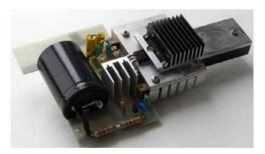
On all the surfaces of the radiators and the transistor that come into contact with each other, there is abundant thermal paste applied. The total cooling surface area is 520 square meters. see. To facilitate the thermal regime of the pass transistor, an additional
