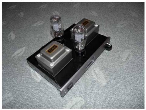
transformers (one for each channel) and kenotrons as rectifiers. Eugene, he the author of the anode voltage stabilizer circuit, advised me to get by with two stabilizers (one for each channel), and decouple the input and output lamps of each channel with a 100 ohm resistor. The argument was that it would be much easier to perform this way, and the currents in the preliminary lamps
